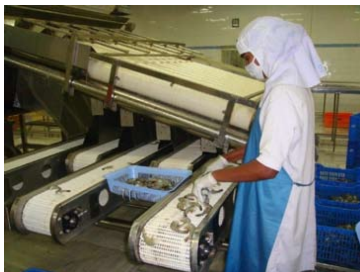
Shrimps being graded according to size (counts) in a sorting equipment
