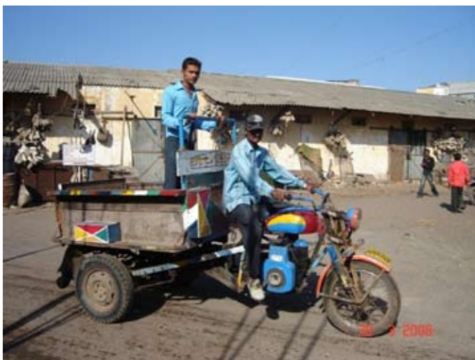
A typical fabricated three-wheeler being in use for operations related to fish transport at Veraval fish market, Gujarat
